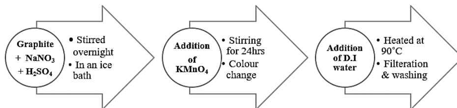
Fig. 5: Schematic flow diagram for synthesis of GO by modified hummer's approach
