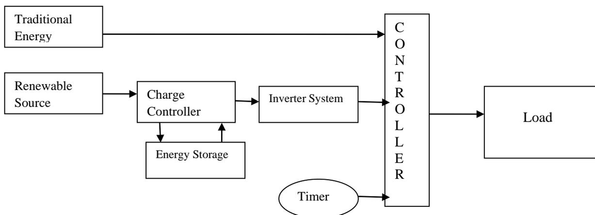
**Figure 1:** Model using the renewable energy and traditional energy controlled by the controller with the help of a timer
