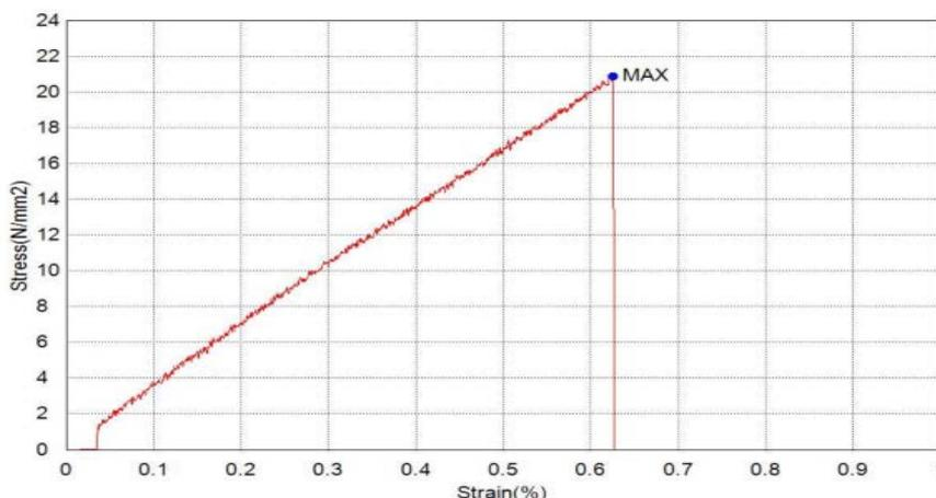
Fig 17: Stress vs Strain graph of Composites A (Bending)
