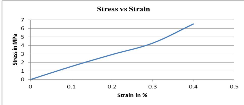
**Fig 14:** Stress vs Strain graph for C composite (Tensile)
