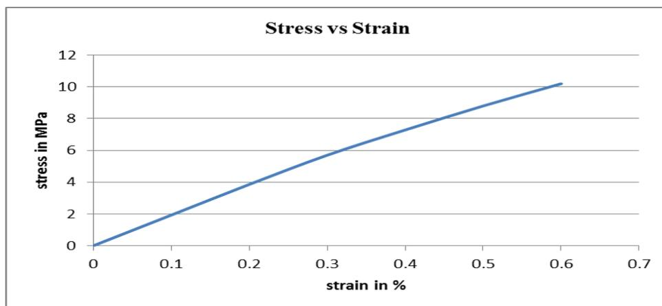
**Fig 13:** Stress vs Strain for Strain graph for B composite (Tensile)
