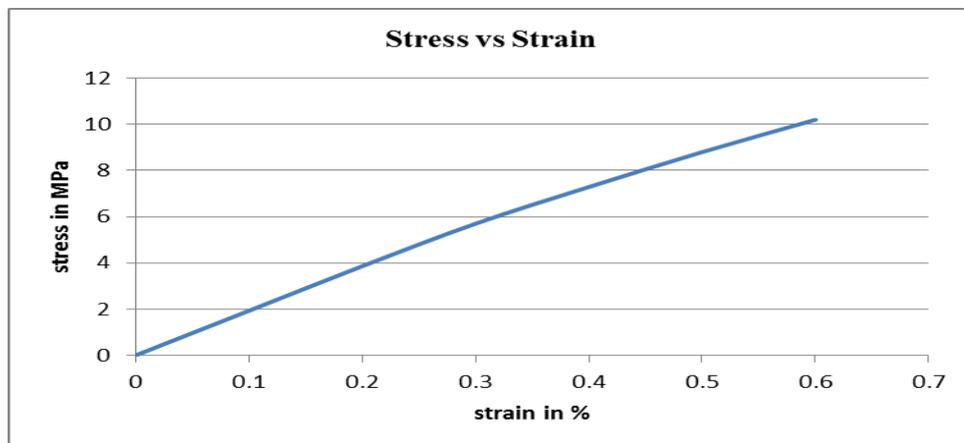
**Fig 13:** Stress vs Strain for Strain graph for B composite (Tensile)
