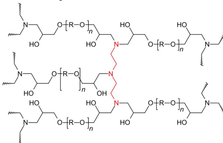
**Fig 3:** Structural Formula of Epoxy
