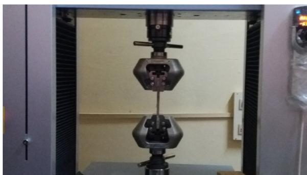
**Fig 7:** Universal Testing Machine **Fig 8:** The arrangement of the specimen in UTM
