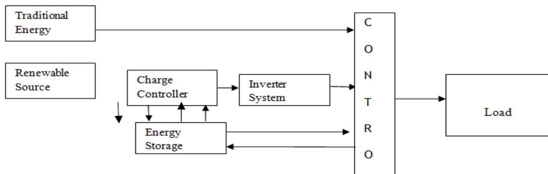
**Fig 21:** Model using the renewable energy and traditional energy controlled by the controller by referring battery voltage
