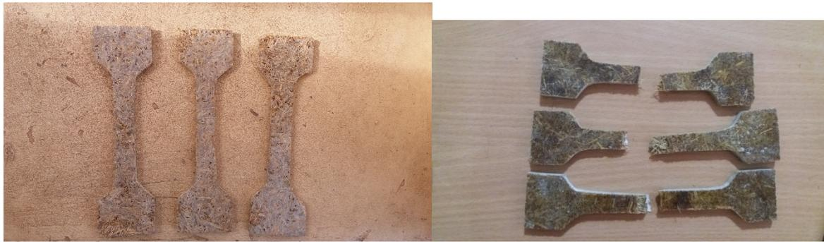
Fig 9: Tensile specimen before and after test
