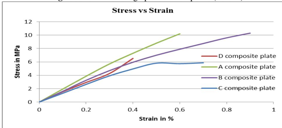
**Fig 16:** Consolidated Stress vs Strain graph of Composites (Tensile)
