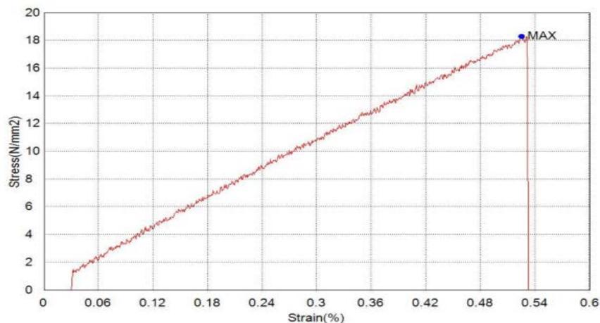
Fig 20: Stress vs Strain graph of Composites D(Bending)
