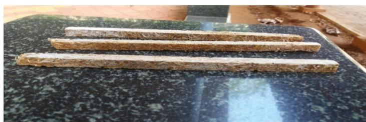
Fig 11: Bending test specimen
