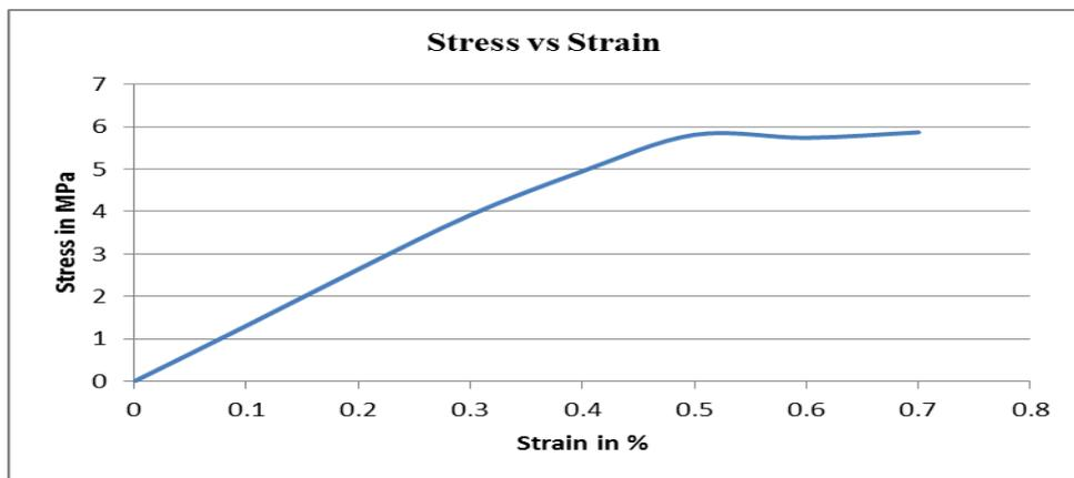
**Fig 15:** Stress vs Strain graph for D composite (Tensile)
