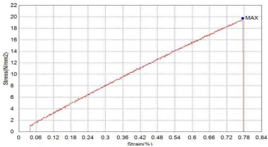
Fig 19: Stress vs Strain graph of Composites C(Bending)
