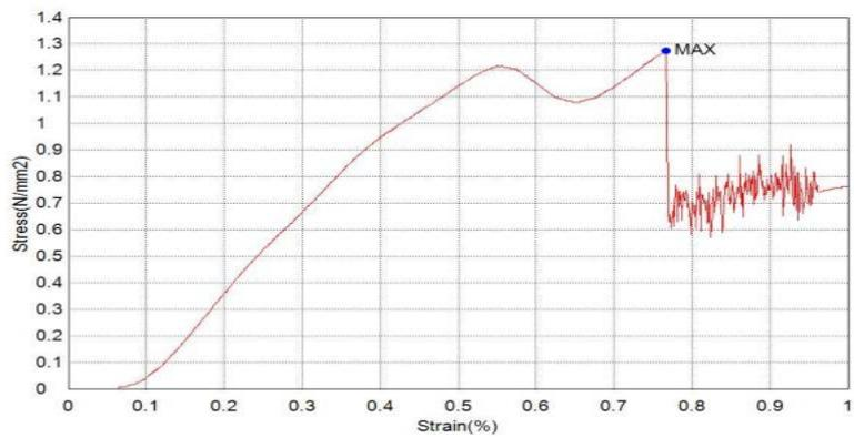
Fig 18: Stress vs Strain graph of Composites B(Bending)
