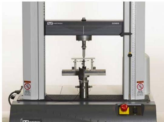
Fig 10: Arrangement for 3 Point bending
