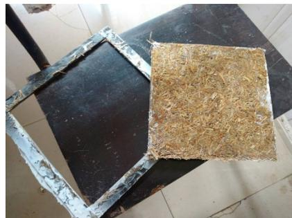
Fig 6: Prepared Composite plate Sample removed from frame
