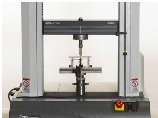
Fig 10: Arrangement for 3 Point bending
