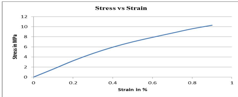
**Fig 12:** Stress vs Strain graph for A composite (Tensile)
