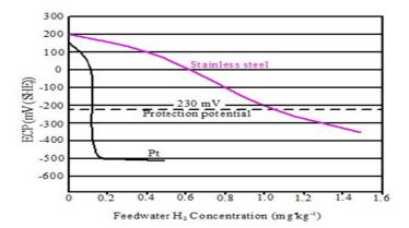
Fig. 3: Variation of corrosion potential of stainless steel as a function of feed water Hydrogen concentration.
